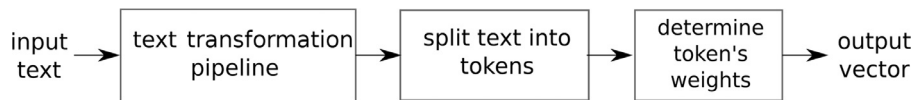
Fig. 1. Generic treatment of input text to obtain the input vectors for the classifier.
